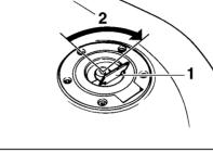
1. Fuel tank cap lock cover 2. Unlock.
